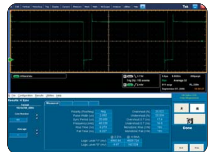
► H Sync Measurement Results (Option VGA).
