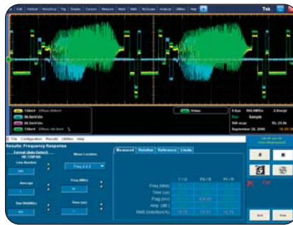
▶ Frequency Response Measurement Input Selections (Option SD and HD).
