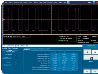
► RGB Transient Response Measurement Results (Option VGA).
