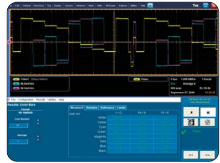
► Color Bar Relative Results Display with Limit Testing Enabled.
