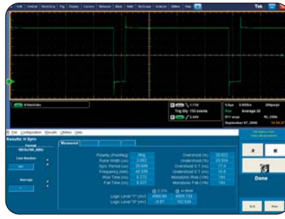
▶ H sync Jitter and Wander Display (Option SD and HD).
