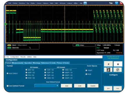
► Signal Format Configuration Menu (Option SD and HD).
